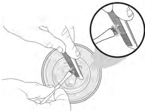
Optimal method for tissue removal - done directly inside the vial
